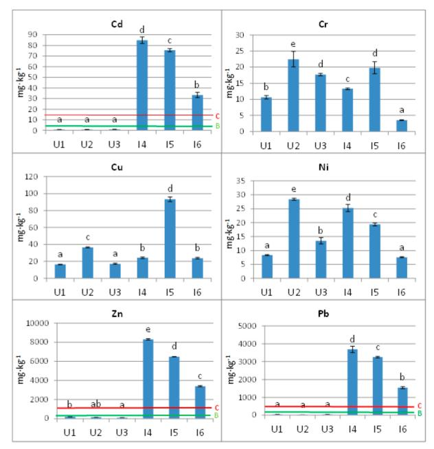
Figure 2. Content of total heavy metals  $[mg \cdot kg^{-1}]$  in soils collected from investigated locations. Lines on the figures present limits elaborated by the Polish Ministry of the Environment for B and C groups. Values marked with the same letters did not differ significantly with  $\alpha = 0.05$  (Standard deviations are presented as plus/minus error bars)
