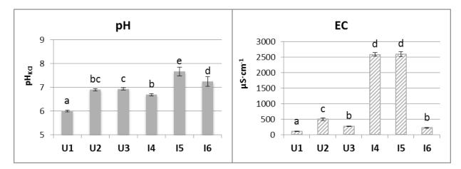
Figure 1. Values of soil pH<sub>KCl</sub> and EC [ $\mu$ S·cm<sup>-1</sup>] marked for investigated locations. Values marked with the same letters did not differ significantly with  $\alpha = 0.05$  (Standard deviations are presented as plus/minus error bars)
