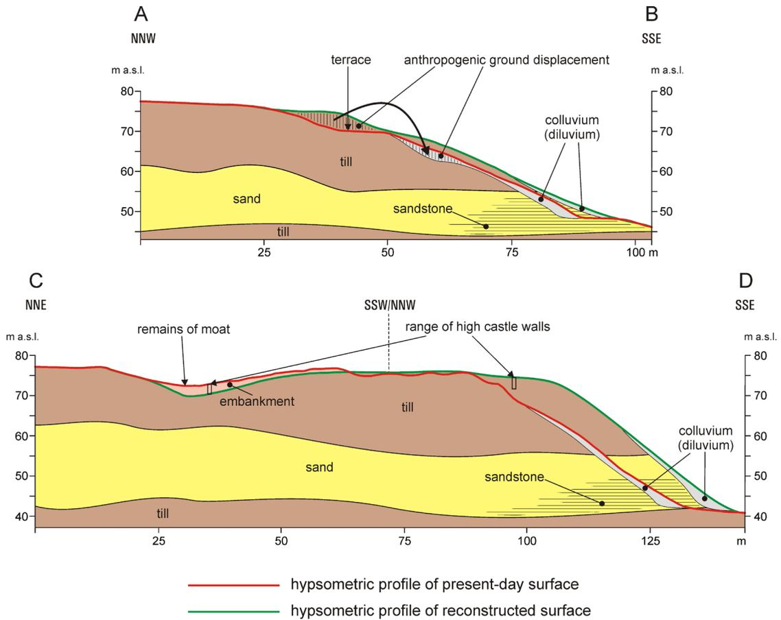
Fig. 10. Model of geological structure and the occurrence of terracing on the south slope of the quasi-peninsular plateau site of the castle at Starogród
