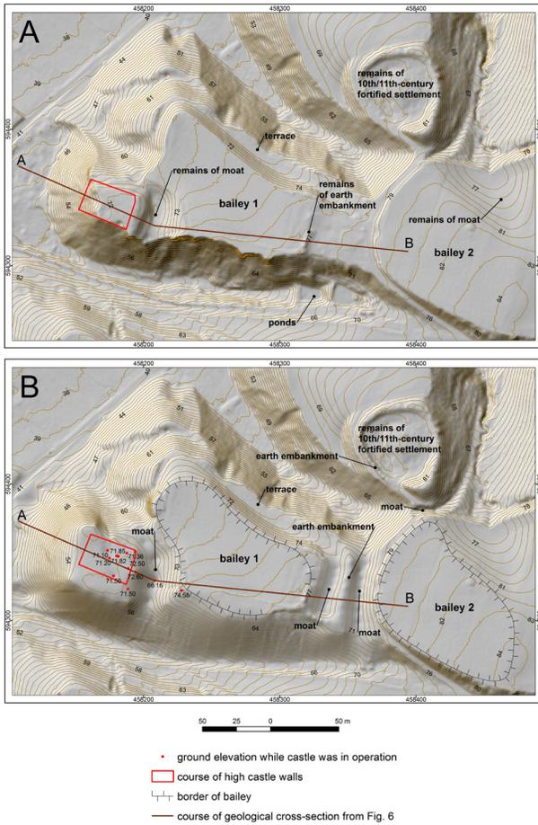
Fig. 4. Attempted reconstruction of the topography of the castle at Unisław: A – digital elevation model of the present-day surface; B – digital elevation model of the reconstructed surface
