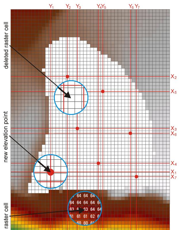
Fig. 3. Method used for modification of the digital elevation model (DEM)
