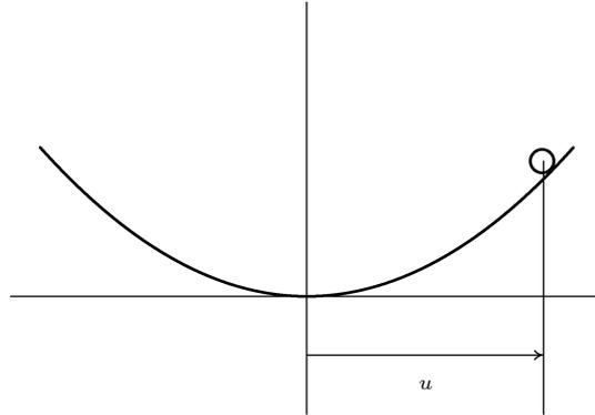
FIGURE 1. A ball-bearing oscillating in a smooth tube bent to produce a restoring force proportional to cube of the displacement
