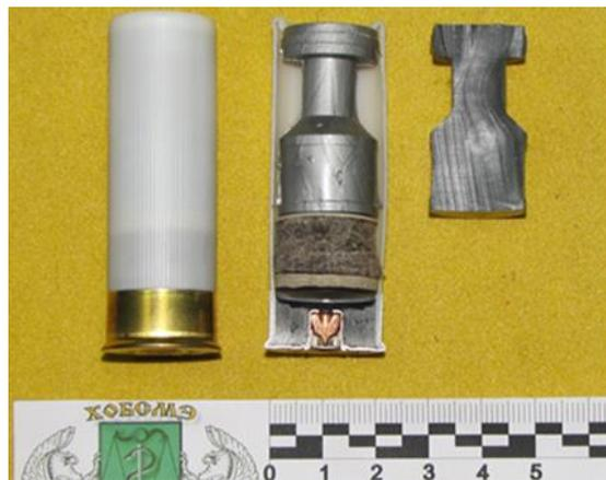
Fig. 2. Picture of the cartridge shock-traumatic (non-lethal) action "Teren-12P" of the 12th caliber and the elastic bullet with which it is equipped
