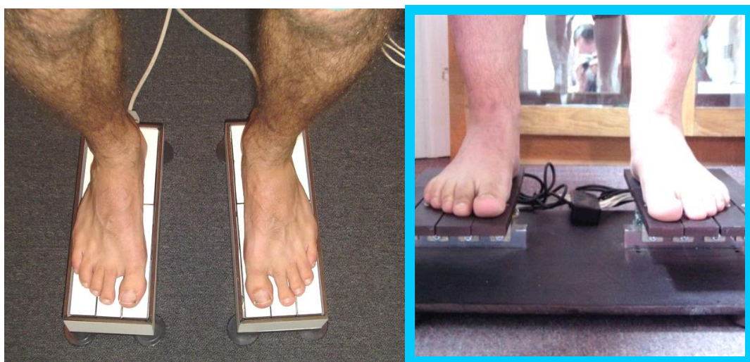
Fig. 2. Position of patient's feet on load cell platforms
