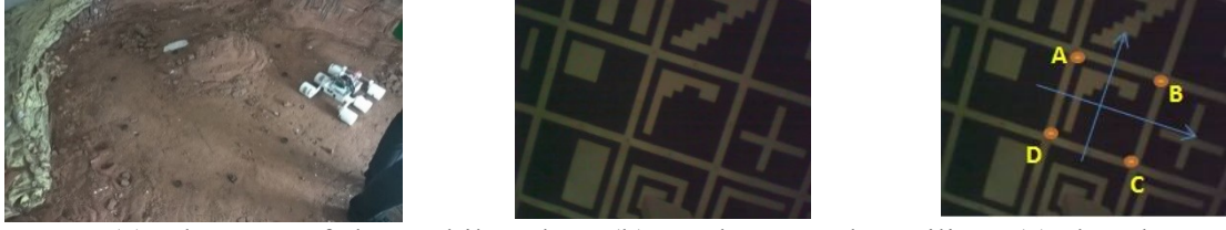
Figure 2 (a) The area of the mobile robot, (b) markers on the ceiling, (c) the photo with coordinates on the marker
