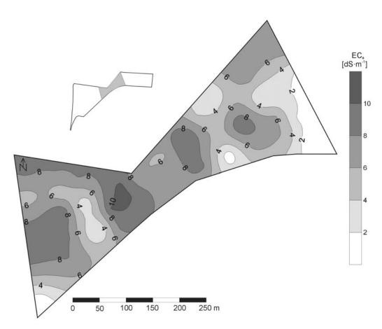
Figure 2. Map of bulk soil electrical conductivity [EC<sub>a</sub>] measured in 0-10 cm layer by TDR method (2009)
