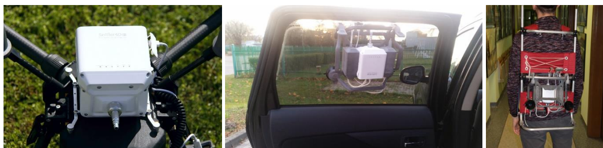
Fig. 4. Integration of the Sniffer4D system with a DJI Matrice UAV(left), with a car (middle) and a pedestrian (right)
