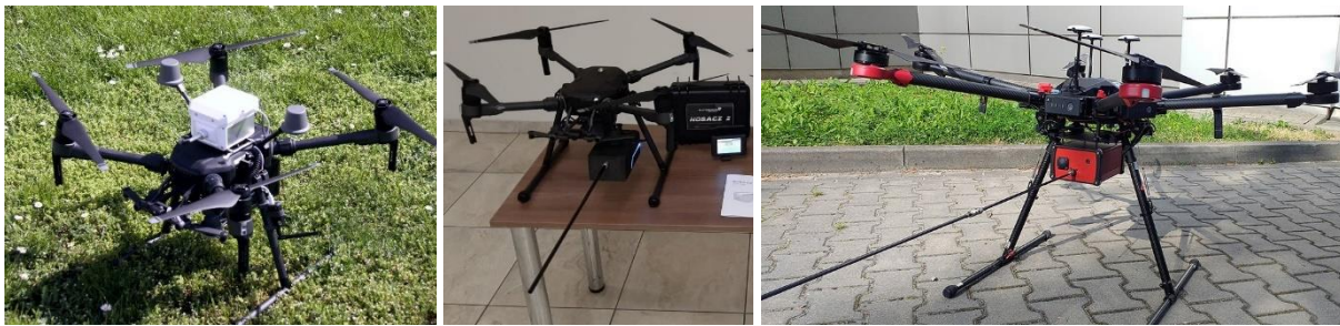
Fig. 3. Mobile air pollution measurement systems integrated with UAV: Sniffer4D (left; photo by: Mieczyslaw Kunz), Nosacz II (middle; source: www.nextron.pl), AirDron (right; source: www.navigate.pl)
