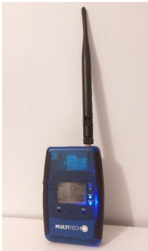
Fig. 5. Compact LoRaWAN mDOT tester from Multi Tech Systems, Inc. used in the field tests.
