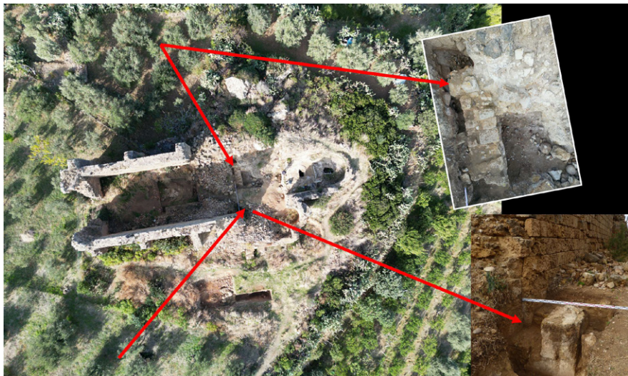
Fig. 18. Santa Maria di Campogrosso. The remains of pillars supporting the chancel wall and the church tower (photo by S. Moździoch)
