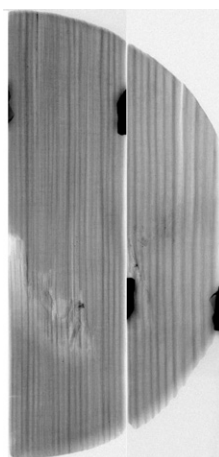
Fig. 5. Radiographic image of the bottom of the stove-built vessel. Visible wood structure and defects of the artefact (dark areas are a metal handle) (developed by B. Miazga)
